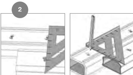
Measure the distance between posts. Center the bottom rail hole pattern within this dimension and cut to length. Place it between the posts and check for a snug fit. Align the top and bottom rail holes and mark the cut length on the top rail. Cut and test fit.
