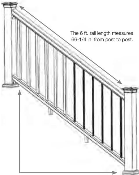
Maximum distance between post sleeves is 56-3/16 inches for a 6 ft. rail.
