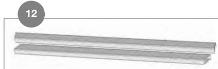
Mark the required stair angle on the ends of each baluster to be used and cut on the top and bottom of each baluster. Ensure that all balusters are of an equal length.
