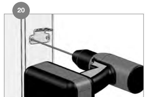
Remove top rail and balusters. Pre-drill the holes with a 5/32 in. bit, angling slightly upward and inward to allow for clearance from the rail when it is repositioned for securing (bracket outline shown for clarity - do not remove the bracket from the top rail).
