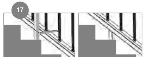
Using an extra baluster, cut two crush blocks to fit the angle and height of the bottom rail from stair treads at the 1/3 and 2/3 points. Secure them to the bottom rail using a quality exterior adhesive.
