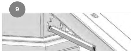
Place the bottom rail between the posts. Using the bracket as a guide, mark the location of the holes.
