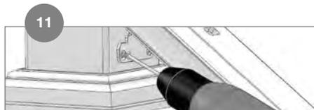
Secure the bottom rail to the post at both ends using the supplied 2 in. screws. Do not over tighten.
