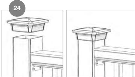
Complete the assembly by positioning and gluing post sleeve caps in place.
