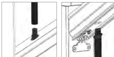
Insert a bottom dagger into the routed holes at each end of the bottom rail. Place two balusters onto the bottom rail, one baluster on each end. Insert a top dagger into the top of the end balusters. Lower the top rail onto the two balusters. Be sure to line up the baluster daggers with the top rail routed holes. Fully engage all baluster daggers into balusters and rails.
