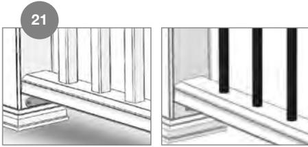
Insert remaining bottom daggers into the bottom rail. Fit all balusters onto the bottom rail.
