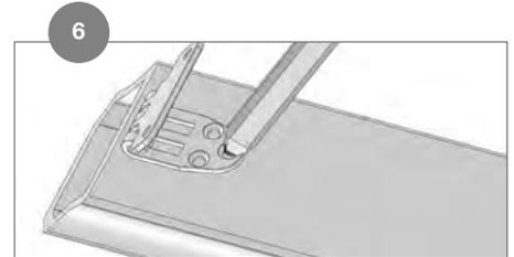
Place the brackets on the flat side of the bottom rail (no holes), and inside the channel of the top rail (with holes), making sure to leave 1/32 in. to 1/16 in. space from the cut edge of the rail. Using the bracket as a template, mark the hole locations.
