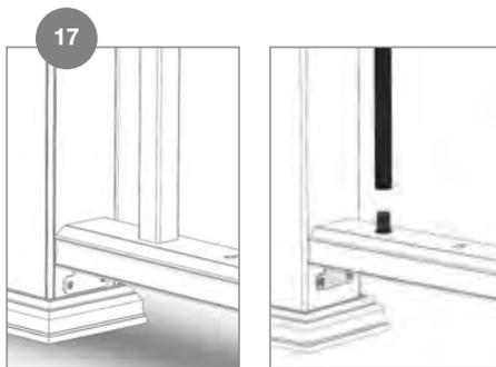
Place two balusters onto the bottom rail, one baluster on each end. Place the top daggers into the balusters.
