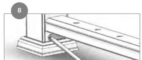
Place bottom rail between posts. Support the bottom rail level and at the desired height using the adjustable crush blocks. Using a tape measure, center the rail on the posts and mark the bracket hole locations.
