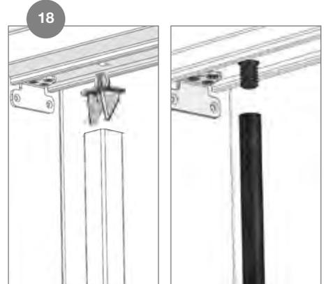
Lower the top rail onto the two balusters. Be sure to line up the baluster daggers with the top rail routed holes until the top rail is fully seated on balusters.
