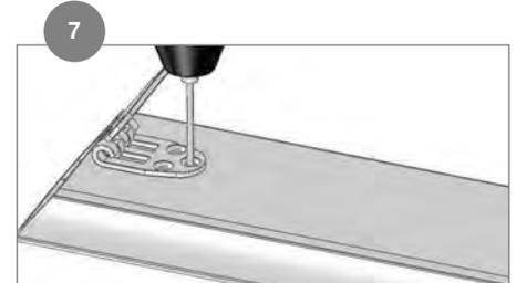
Pre-drill holes with a 5/32 in. drill bit (bracket shown for clarity).
