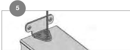
Secure the bracket with supplied 1 in. screws. Do not over tighten.
