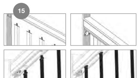
Insert remaining bottom daggers into the bottom rail. Place all balusters on bottom stair rail. Working from one side to the other, insert top daggers into remaining balusters. Slowly lower the top rail in place, aligning baluster daggers with the top rail routed holes. Fully engage all baluster daggers into balusters and rails.
