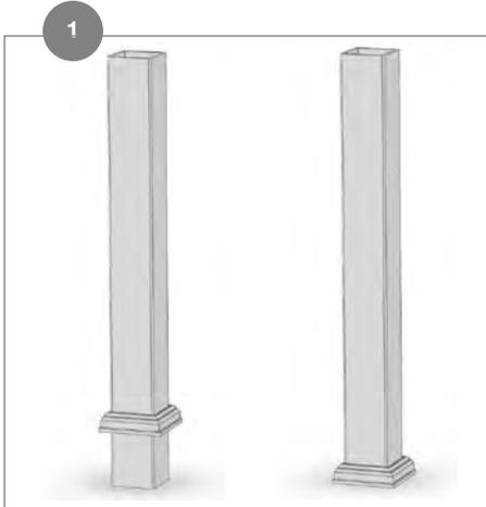
Cover 4x4 posts or Fiberon surface mount brackets with post sleeves and verify the spacing. Posts should be plumb in both directions. Place post sleeve base mouldings over the post sleeves and slide it down to the deck surface.
