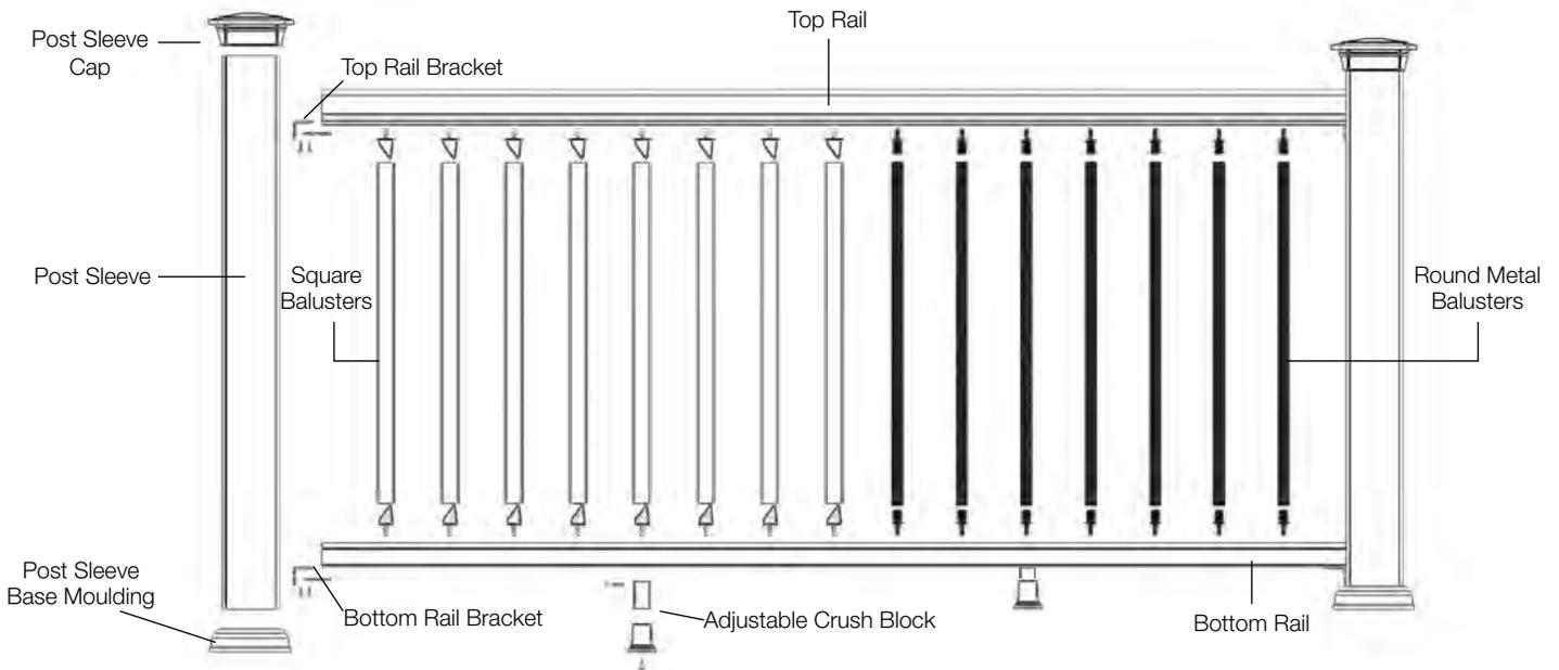
*Note: Rail lengths will vary slightly due to the manufacturing processes. Make sure rails are cut to the correct length, and the hole pattern is centered between posts before securing.*
