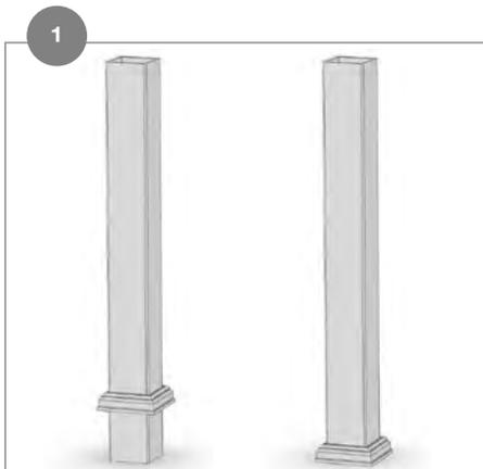
Install 4x4 posts in the pre-determined locations. Cover with post sleeve and verify spacing. Posts should be plumb in both directions. Place post sleeve base moulding over post sleeve and slide it down to the deck surface.
