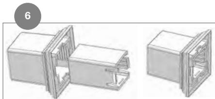
To assemble the adjustable crush blocks, push the center up through the base, making sure that the compression wings align with the ridges inside the core. Insert until the first "click" is heard. If the center is inserted too far, it can be pushed through completely.
