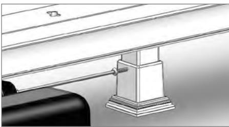
If not previously extended, extend the adjustable crush blocks to the final height, making sure the rail is level. Lock the block in place by drilling a 5/32 in. hole into one face and securing it with the supplied 3/4 in. screws. Do not over tighten.
