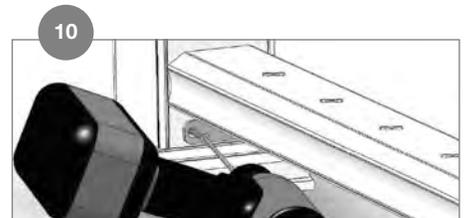
Secure the bottom bracket and rail to the post using the supplied 2 in. screws. Do not over tighten.
