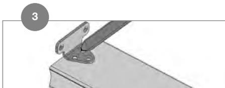
Flip the bottom rail so that the pre-routed holes are facing downward. Center the bracket at each end of the bottom rail. To help ensure a snug installation, allow 1/32 in. to 1/16 in. clearance between the bracket "wing" and end of rail. Mark hole locations.
