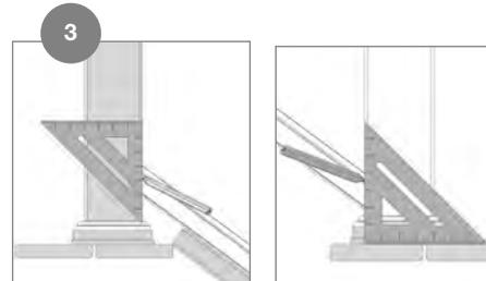
Mark the angle on the bottom rail using the inside of each post. Cut the bottom rail to the required length and check for a snug fit.
