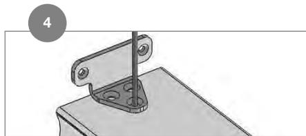
Pre-drill holes in the bottom rail using a 5/32 in. bit (bracket shown for clarity).
