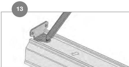
Flip the top rail so that the pre-routed holes are facing upward. Center the bracket on the rail. To ensure a snug installation, allow 1/32 in. to 1/16 in. clearance between the bracket "wing" and the end of rail. Mark hole locations.
