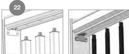
Insert remaining top daggers, either into the balusters or into the top rail. Working from one side to the other, slowly lower top rail in place. Fully engage all baluster daggers into balusters and rails.
