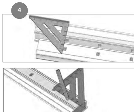
Measure the distance from the cut bottom rail end to the first hole. Transfer the dimension to the top rail; then, align both rails together.
