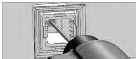
Find the 1/3 and 2/3 point on the bottom for the two adjustable crush blocks provided (white railing only has 1 adjustable crush block for centered placement). Pre-drill a hole with a 5/32 in. bit. Secure the adjustable crush blocks with the supplied 3/4 in. screws. Do not over tighten.
