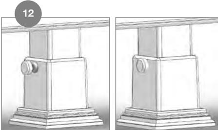
Cover the exposed head of the screw with the supplied screw cap.
