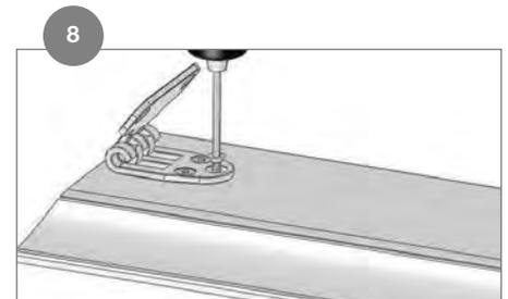
Secure brackets with supplied 1 in. screws. Do not over tighten.
