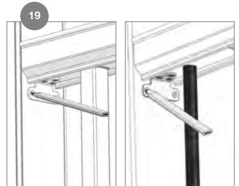
Ensure the top rail is level. Mark the top rail bracket hole locations.
