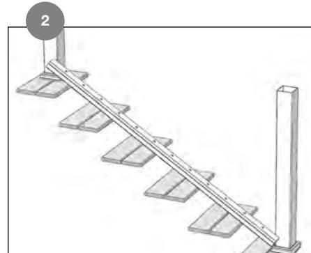
Center the hole pattern between the posts, allowing a minimum 2-3/4 in. from rail end to routed baluster dagger holes.
