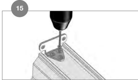
Secure the bracket with supplied 1 in. screws. Do not over tighten.
