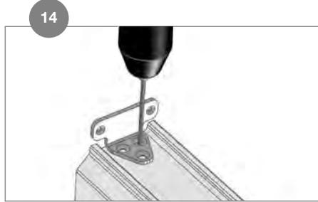
Pre-drill holes using a 5/32 in. bit (bracket shown for clarity).
