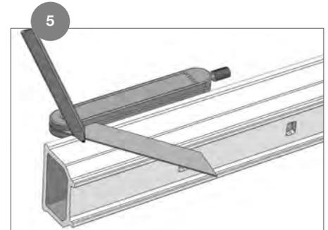
Transfer the cut angle and cut top rail to length.
