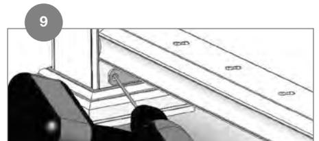
Pre-drill the holes with a 5/32 in. bit, angling slightly upward and inward to allow for clearance from the rail when it is repositioned for securing.
