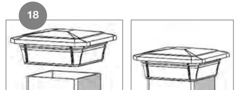
Complete the assembly by positioning and gluing the post sleeve cap in place with a quality exterior adhesive.
