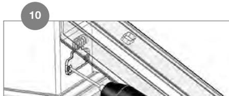
Pre-drill the holes with a 5/32 in. bit, angling slightly upward and inward to allow for clearance from the rail when it is repositioned for securing (bracket and rail outline shown for clarity.)
