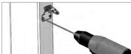
Once fully seated, mark the location of the bracket holes. Remove the top rail and pre-drill the holes with a 5/32 in. bit, angling slightly upward and inward to allow for clearance from the rail when it is repositioned for securing (bracket outline shown for clarity - do not remove from top rail.)
