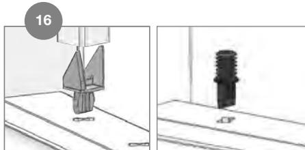
If required, trim the balusters to the desired length. Then insert the bottom daggers into the two outermost dagger holes.
