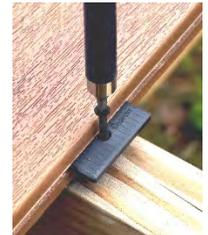
*The Phantom universal deck clip is 38 mm wide and is designed to completely cover the joist to further enhance the hidden fastener aesthetics. Also, please note that Phantom Universal Hidden Deck Fasteners provide a 5 mm gap between each decking board.*
